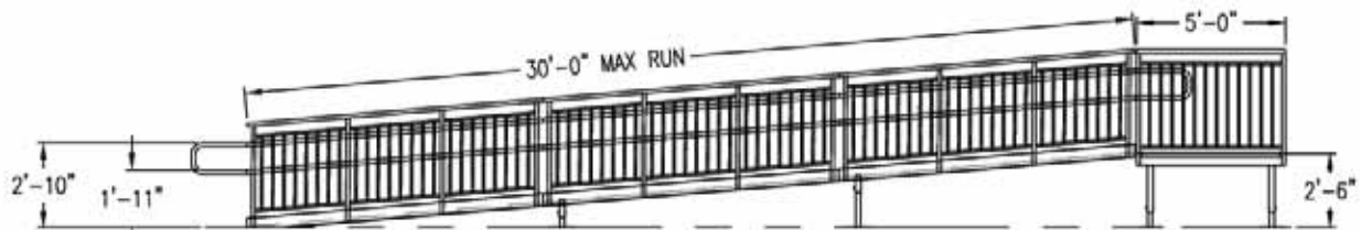
①-C-C 2 ELEVATION VIEW: 42/34/23 VP ALUMINUM ACCESS RAMP SYSTEM
