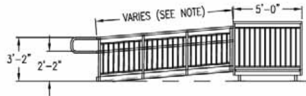
C-C 2 ELEV VIEW: 38/26 VP ALUMINUM ACCESS RAMP SYSTEM NOTE: TO USE 38/26 VP, MAX RUN OF RAMP SYSTEM=30'-0"
